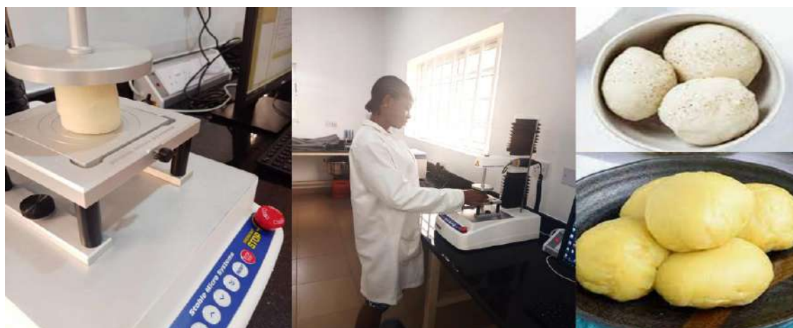
Figure 15: Mid-throughput protocols for profiling textural properties of RTB products with texterometer (ready-to-eat cassava fufu and Eba)
