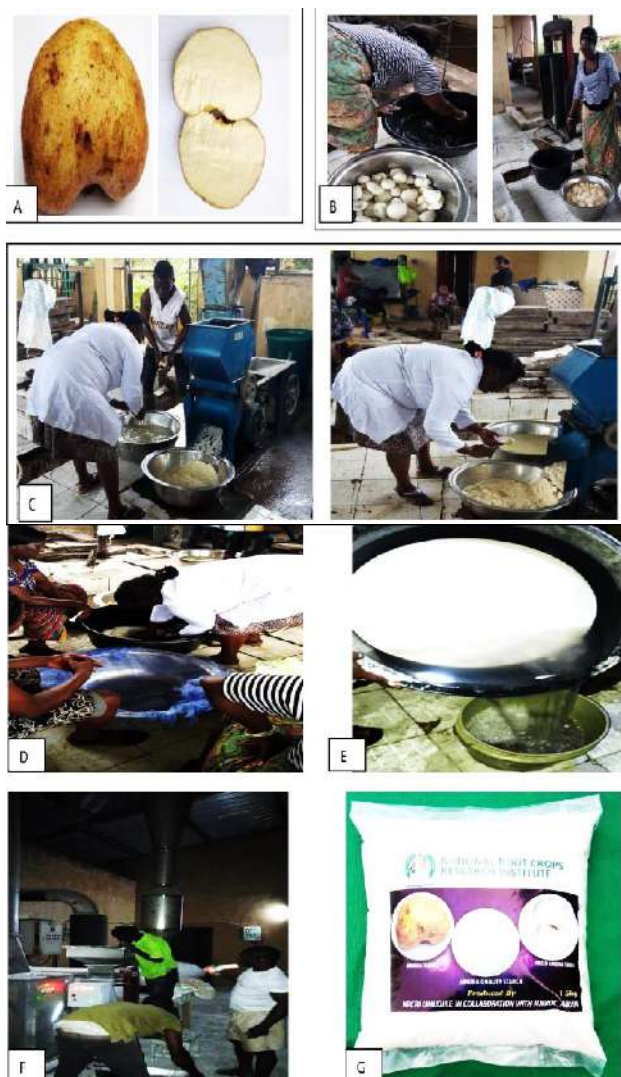
Plate 11: Photographs of some operational steps in amora starch extraction. A = Fresh amora tuber, B= peeled, washed amora tubers steeped in water, C Grating and sampling of amora mash (pulp), D = Multiple washing of pulp to free amora starch, E=decanting washed wet amora starch cake, F= flash drying of wet amora starch cake and G = packaged quality amora starch
