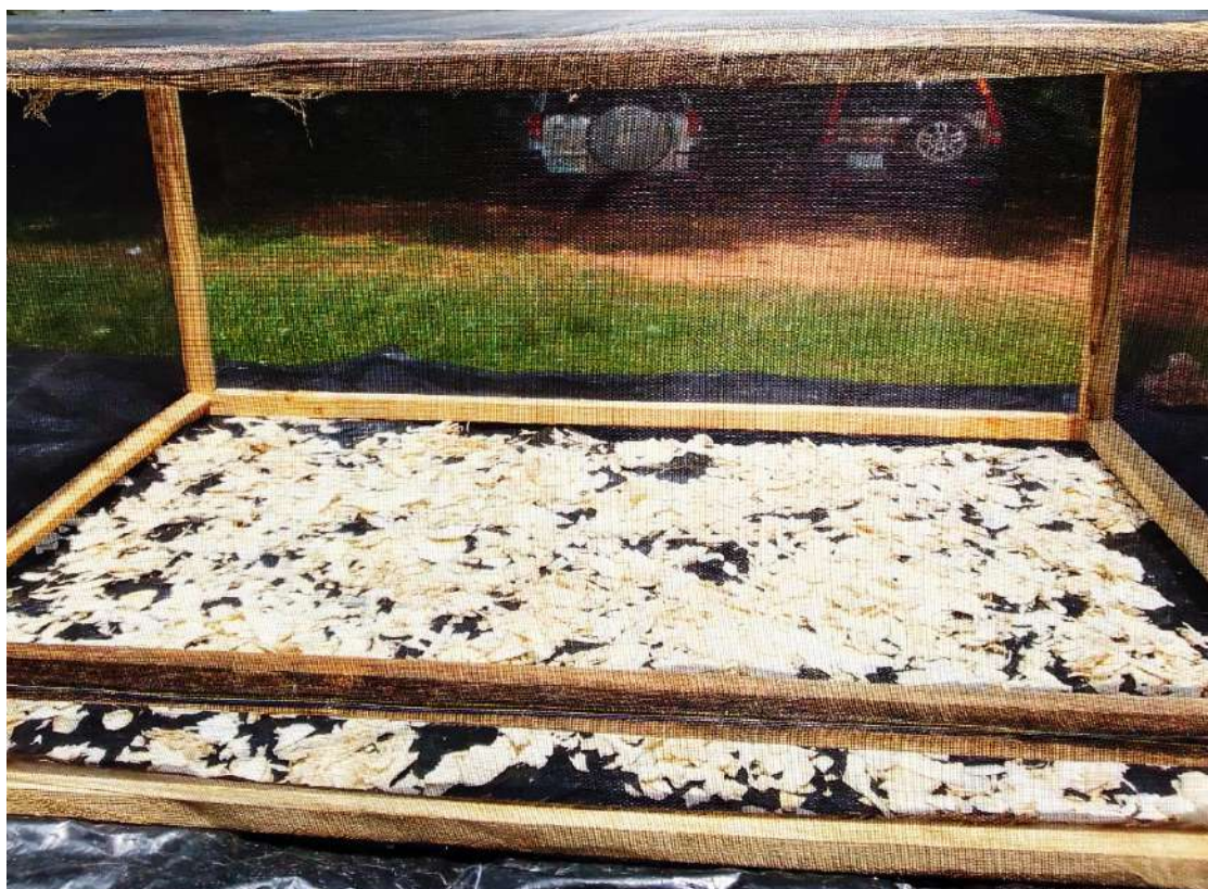
Plate 9: Sun Drying using net tunnel: Net box tunnel (solar dryer) developed to dry food material with acceptable microbial load according to NAFDAC and SON standards
