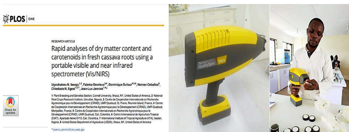
Figure 14: Protocol for the use of Near Infra-red spectrophotometer for predicting of cassava dry matter content, carotenoid starch, amylose and total titratable acidity
